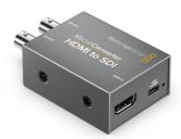
Take the HDMI output from laptop computers or consumer cameras and convert it to SDI for use with broadcast switchers, routers, monitors and more! The multi rate 3G-SDI automatically switches between all SD and HD formats up to 1080p60. You get 2 SDI outputs, support for Level A and Level B equipment, and power over USB!
